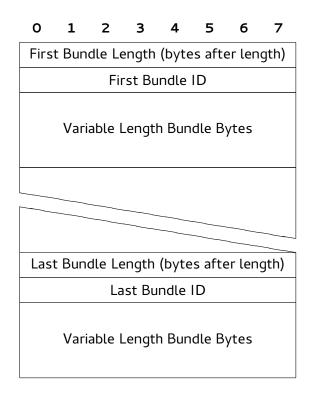
**Bundle Length**: This byte specifies the length of the bundle excluding the length byte. A bundle that has 2 bytes of payload will have a length of 0x03 due to the bundle ID byte.
